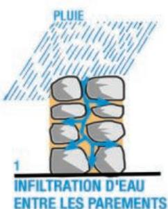
1 INFILTRATION D'EAU ENTRE LES PAREMENTS
